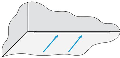
Drain positioned against the short wall.
